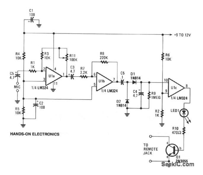
This circuit can cause a cassette recorder to automatically turn on and record when a sound or noise is present. Another use, is when the sound-activated switch is used to turn on a cassette player so that it operates as a burglar-alarm detector and sounder.
